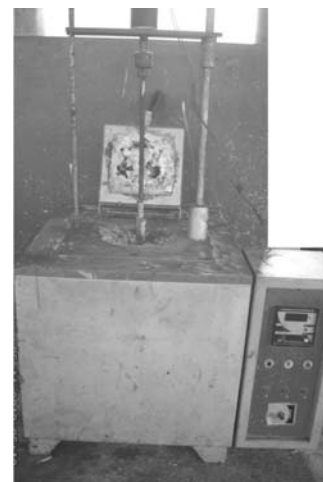
Fig.2. Induction furnace with stirrer
